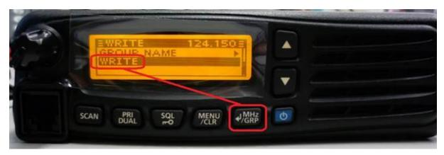
Use the Up/Down Keys to Choose YES (it will be filled in when selected) and then Push MHz/GRP to Lock it into Memory.
