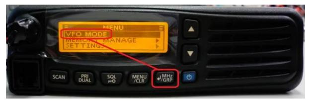
Change to the Frequency you are wanting to enter into Memory with the Up / Down Keys. First Set the MHz side then KHz side (by Pushing MHz / GRP Key):
