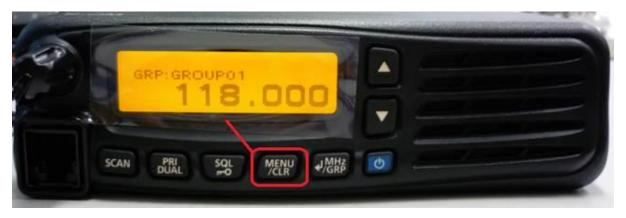
Confirm VFO MODE appears at the top of the Display and Push MHz / GRP Key:
