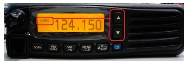
2. Push MENU/CLR Key to enter the Menu and scroll down with the Up/Down keys to Memory Write. Push MHz/GRP Key to enter:
