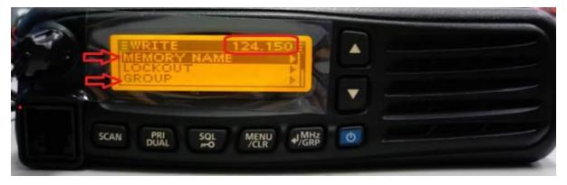
Scroll down with the Up/Down keys to WRITE and Push MHz/GRP Key to enter the mode.
