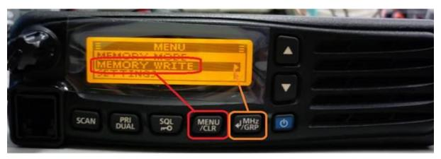
From here you can enter the <u>Memory Name</u>, <u>Lockout</u> (Scan) and <u>Group</u> – Channel Location sections. Confirm the frequency to be programmed across the top of the display:
